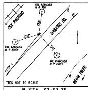
₽ STA. 32+53.75 CBP 6 IS A CAPPED IRON ROD SET IN GROUND WEST OF PAVEMENT EDGE NYSPCS CENTRAL ZONE NAD83 2011 N: 1526473.622 E: 1068345.311
